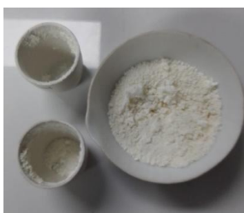
Fig. 1. Image of the ZnO nanoparticles obtained from the green synthesis.
