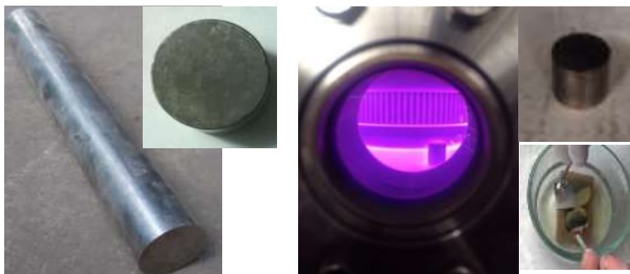
Fig. 1 (a) Cutting of AISI 431 steel samples, (b) plasma nitriding, (c) electrolytic etching of samples
